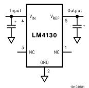
\*Optional, Recommended for improved transient response and input noise reduction.
